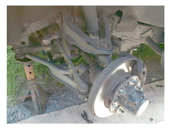
2. Remove drop link, mine seemed to have worn the hole in wishbone slightly to big, so as you will see I have put very thick washers either side of wishbone to stop nut and rubber pulling through in the future (I hope). I recently bought this wagon the link must have been well gone weeks before. I removed the rubber lower bump stop, just 1 x 10mm nut from underneath with deep socket, to allow more access.
