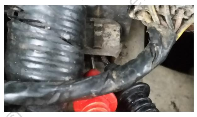
Then set your multimeter to Ohms, once on this setting it should measure 100 ohms or close to, if it doesn't then you're No1 injector is faulty and needs to be replaced
