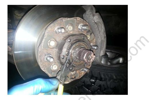
Once that has been removed, slide off the threaded washer and 2 rings behind it and make a note of the order and position they were in before removed ready for re-assembly
