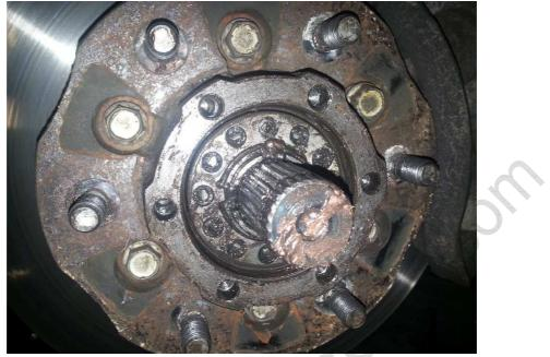
Once you have removed the above, you will then be able to use the head of your screwdriver in one of the holes in the threaded washer that holds the outer bearing in position, turn ant-clockwise and remove.
