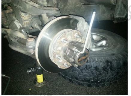
Once it is off you will then need to remove a circlip and some other washers held on the shaft.
