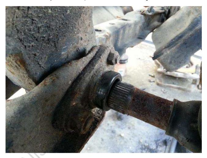
Now you need to turn the bar towards the opposite side of the truck by one maybe two splines, that is why i said draw the line it acts as a reference point to where the splines originally sat.
