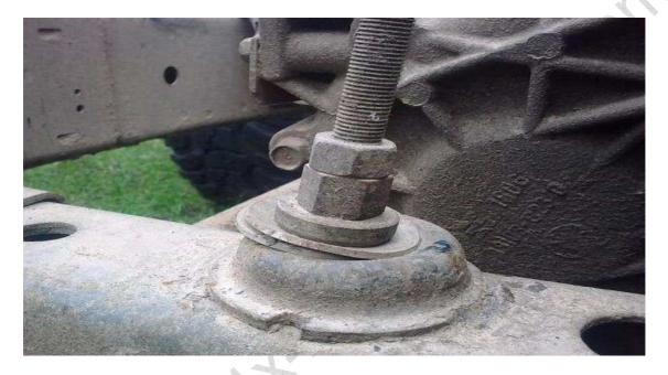
Then remove the adjusting bolt
