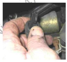
5) Remove the sensor using the 26 or 27mm long socket on the end of the  $\frac{1}{2}$ " drivers.
