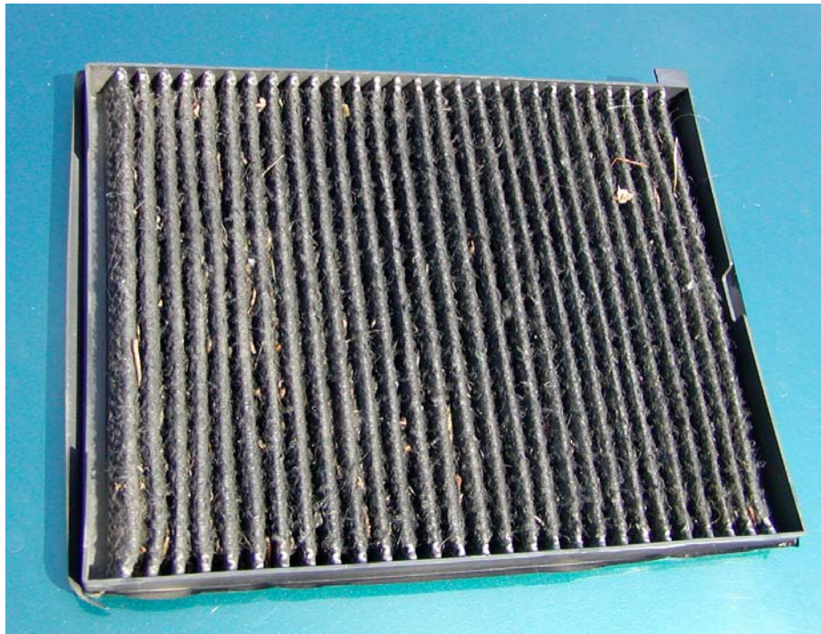
One blocked Filter
