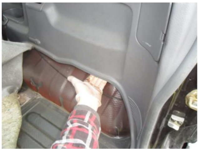
First undo the screws on the boot trim at the entrance then pull the plastic clips around the right side panel so you can pull the carpet out. (see picture above)
