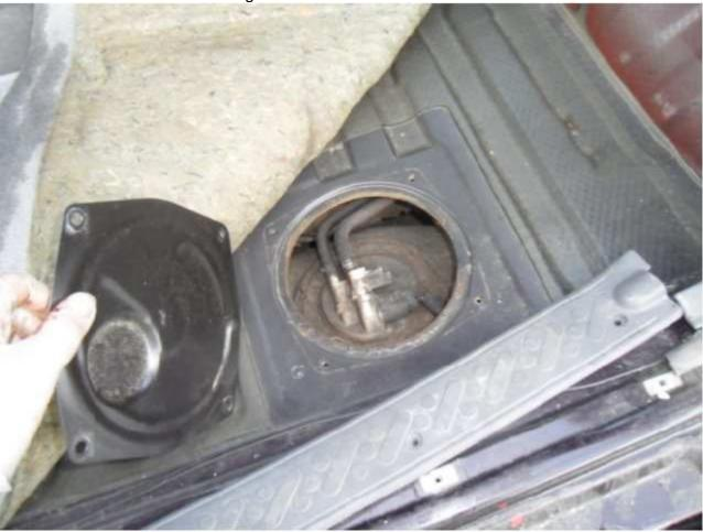
Next make sure the fuel line hose you bought fits the fuel tank supply and return nipples. Remember they are two different sizes.
