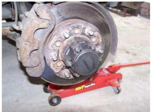
Once removed you will be able to prise the hub away from the wheel disk, I used a rubber mallet to break the seal, but don't hit it too hard, you don't need too.
