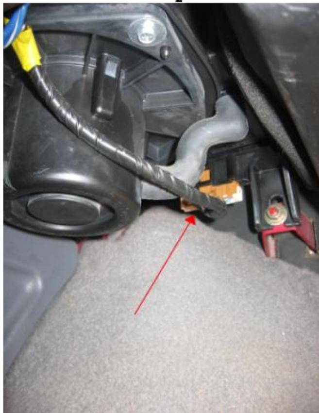
*Undo the two screws and withdraw the resistor downwards, then remove the plug connector by squeezing the top of the brown retaining clip, you have now removed the defective heater blower resistor. See pic 3& 4:-*
