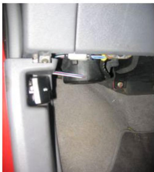
*The part you need to replace is located almost up against the bulkhead and is secured by two screws, if you are a bit of a contortionist you should be able to get at them without removing anything else, eg. glove box. see picture 2:-*
