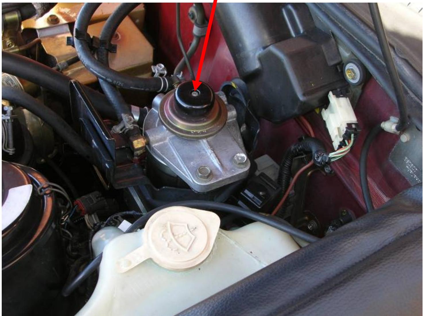
Once firm you can start your engine and run. After a short run prime filter again to remove any excess air that might have appeared and check for any leaks.
