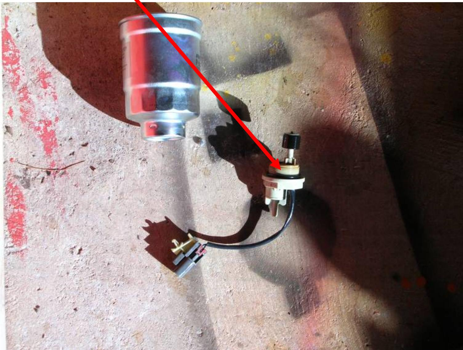
Once screwed on to new filter it is ready for re-installing back into engine bay.
