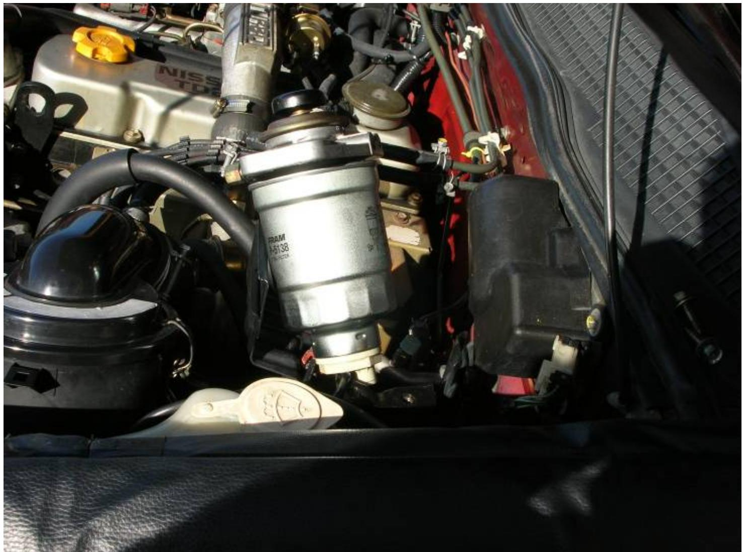
Pour Diesel from the filter into your clean container for temporary storage.
