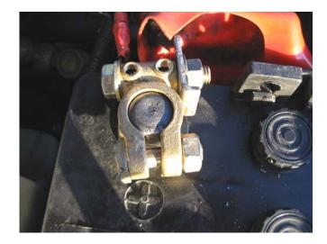
Assemble the post terminal 8mm nut and bolt as pictured above. taking care regarding the natural lie of the cable and vibration of the engine, also this connection will be required to pass 100's of amps on starting, therefore the mating surfaces need to be as large as possible,
