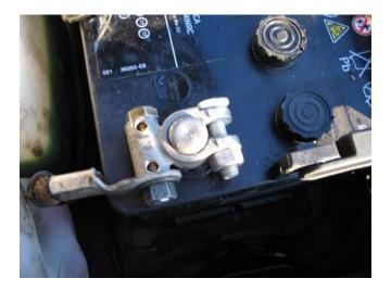
Remember to unlock all the doors before disconnecting the battery and grease up the battery terminals afterwards to protect them from corrosion.
