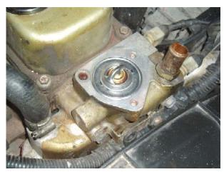
Wire brush the three bolts and coat in copper grease. Use a new gasket and bolt back up loose and then a little at a time on each bolt, don't over tighten!
