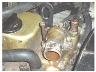
Remove old stat and clean up any old gasket remnants from the head and the stat housing.
