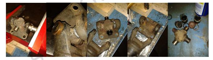
Time to clean all the surfaces up as well as the circlip rebate and a little bit of grease to help the cups slide back in.
