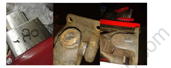
It is also important to remember to mark the saddle and shaft so that they go back where they came from as the shaft would have been balanced when originally built.
