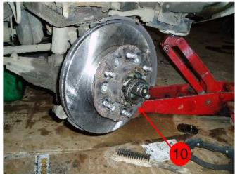
Withdraw outer wheel bearing 10
