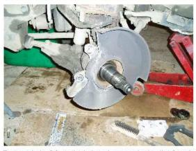
Carefully pull hub and disc assembly from axle, this should take no more than hand force to remove.
